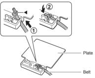
**2** Align the flat surface of the plate with the electronic flash and wrap the belt around the flash (①). Insert the other end of the belt firmly into the plate (②).
